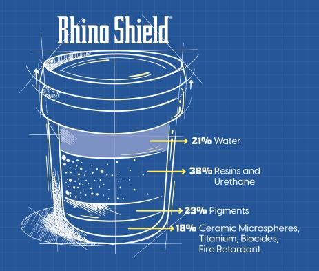
Rhino Shield is exceptionally thicker (8-10 times more) than latex paints. This helps protect the substrate against abrasion and aids in soundproofing your home. While the coating is thick, it doesn't hinder the look and feel of your home's surface material. Wood and metal alike will retain their aesthetic and texture.
